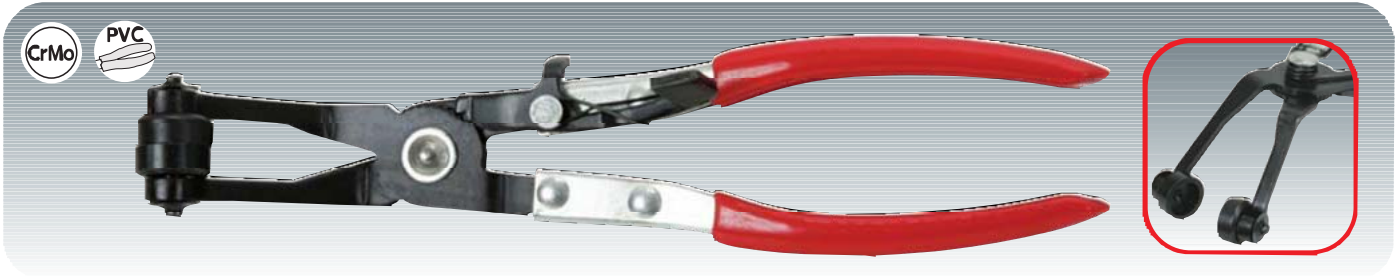
Hose clamp pliers 45° angled, ratchet locking mechanism, swivel jaw spring (recessed/slotted) for self spanning clamps
